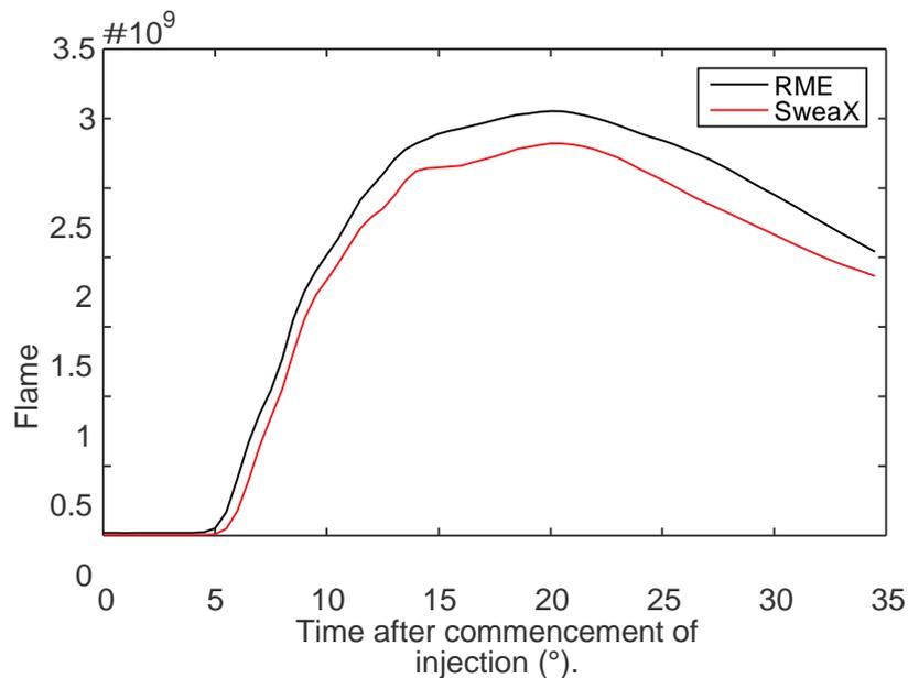
**Figure 6:** Flame intensity is a measure of the amount of soot formed during combustion. The result shows that soot formation is reduced with SweaX compared to RME.
