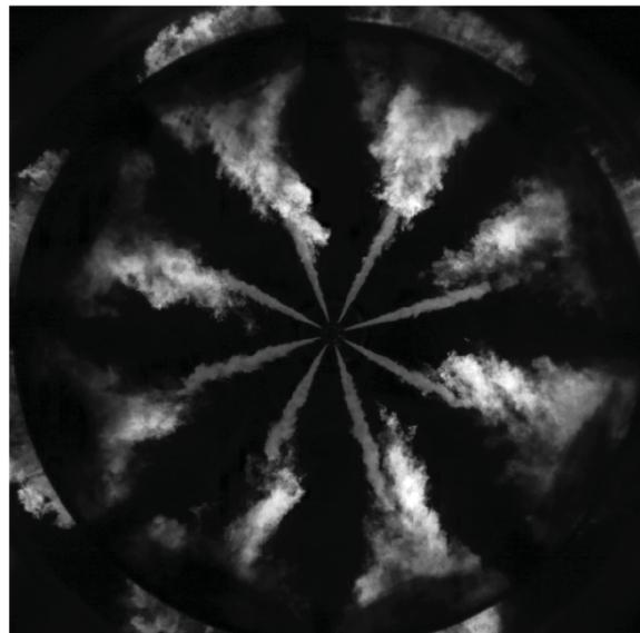
**Figure 2:** Camera view of the combustion chamber. All regularly shaped fuel sprays spread from the centrally mounted injector. The lighter, irregular areas at the end of each spray are flames.
