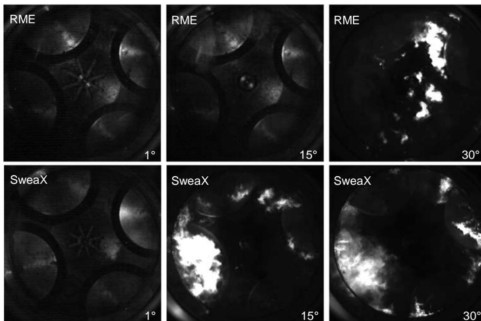
**Figure 3:** Figure 3 provides an example of the ignition process when the two fuels are injected in conditions equivalent to cold start in winter temperatures. The numbers in the bottom right-hand corners show how many degrees the crankshaft has rotated following commencement of injection. SweaX ignited  $15^\circ$  after commencement of injection, while RME ignited later.
