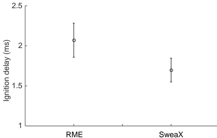
**Figure 4:** Ignition lag, or ignition time, is the time that passes between the commencement of injection and the fuel’s self-ignition in the cylinder. SweaX provides a quicker, more stable ignition process.
