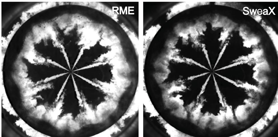
**Figure 5:** Flame brightness or intensity provides a measure of the amount of soot formed during combustion. We see that pure RME has a higher intensity and thus produces more soot than SweaX.
