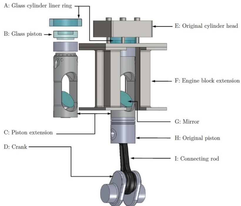
**Figure 1:** Schematic diagram of the optical access fitted to the test engine.
